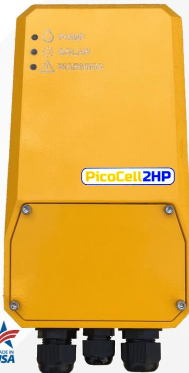
One easy to install, universal controller can power motors, pumps, compressors or other inductive loads regardless of whether it is single or three phase AC, 50 or 60Hz, 120 or 230Vac. Power any 1/3 – 1 1/2 HP motor, and up to 2HP three phase. Designed to handle remote off-grid installations, the all aluminum chassis is IP66 rated for harsh outdoor environments and can operate in high temperatures, humidity and corrosive environments.
