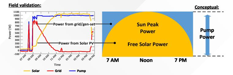
PicoCell with optional Power Blending seamlessly blends energy between a solar array and the power grid. It is ideally suited for applications that require 24/7 or some night time operation, particularly in areas with high power costs. The combination of the PicoCell controller and the optional Power Blending Controller™ represents a cost effective way to intelligently supplement solar power with controllable night time operation, without the expense of adding batteries.
